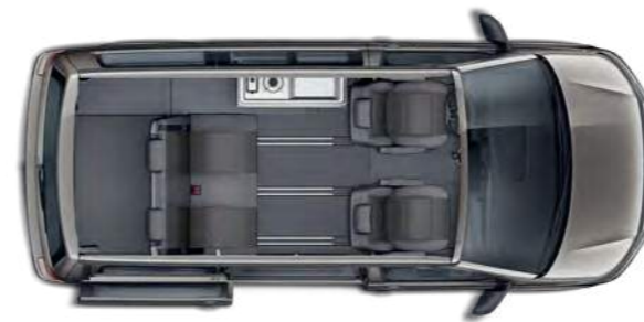
California 6.1 Beach Camper with sliding rear door on the right, mini-kitchen, four seats, stowage areas and folding bed extension.
